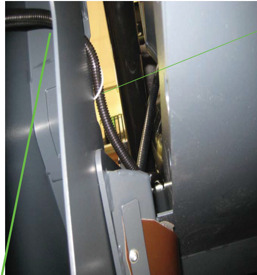
Power cable to rear light/indicator, left Fix cable with cable ties
